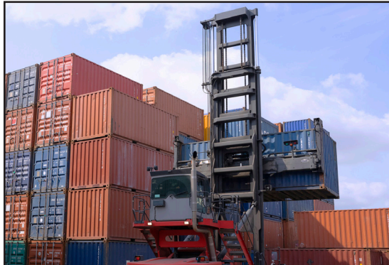
Side loader at a terminal port whose chains were failing prematurely.
