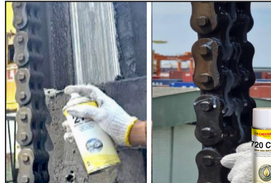
Cleaning with 274 Industrial Degreaser and lubricating with 720 CCG with diluent.
