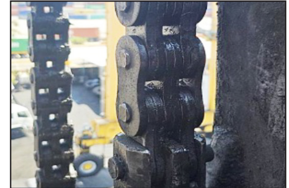
After using 720 CCG with diluent for 6 months, there was minimal corrosion or detectable wear.
